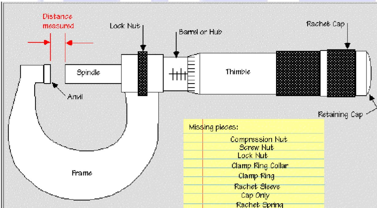
Note: To measure the **wall thickness** of a tube, the anvil should be rounded in order to fit snugly against the inside wall of the tube.
