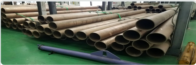
CONFIRMED C70600 PIPE INVENTORY
